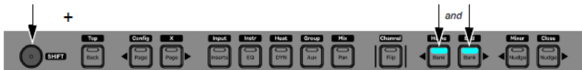
S1 switches to enable Folder Track Multi-Master Mode
