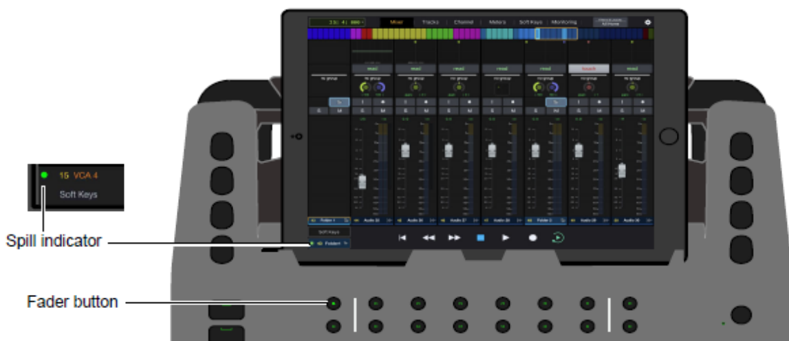
Spill indicator in the Control app and the Fader button on the Dock
