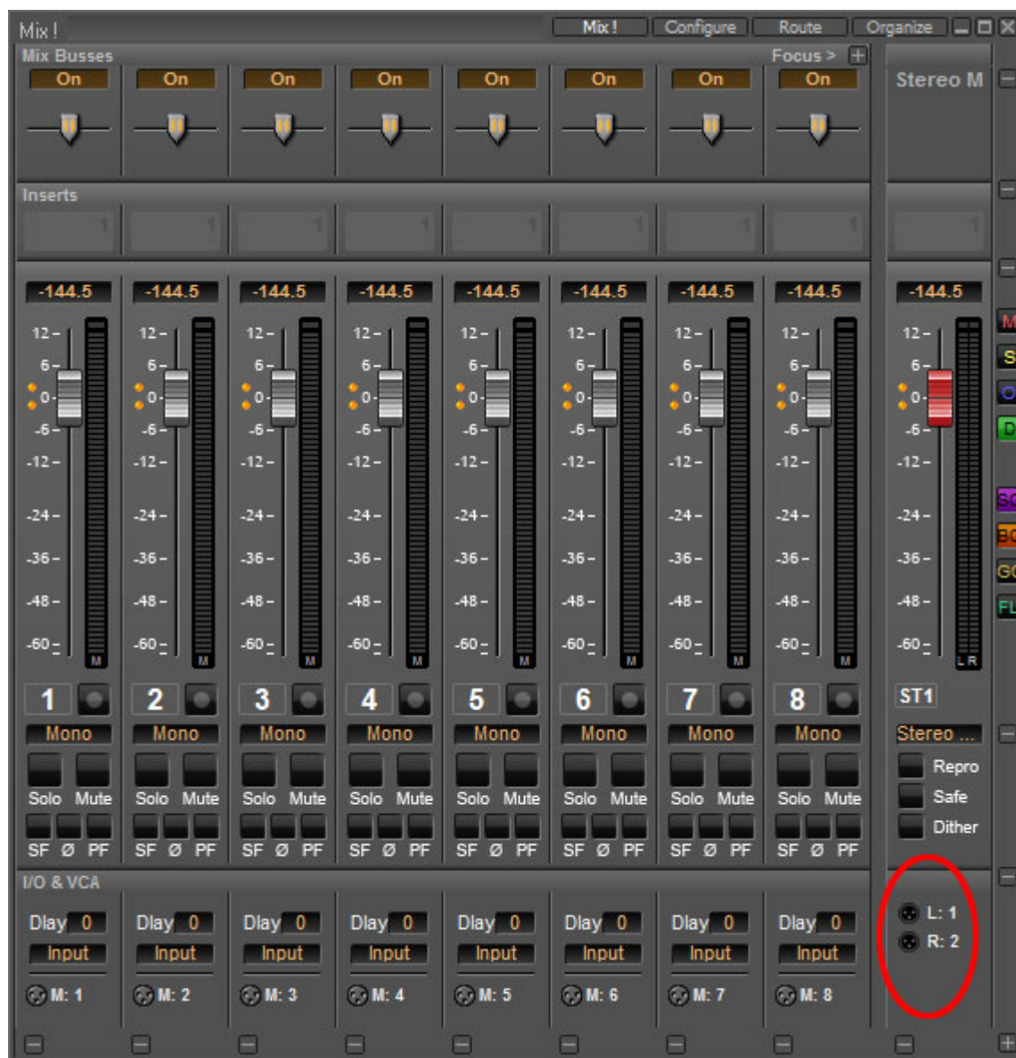
Default Mixer with Output Routing Circled
