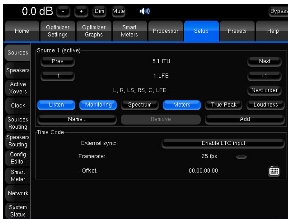
Sources of the MC model (with SmartMeter)
