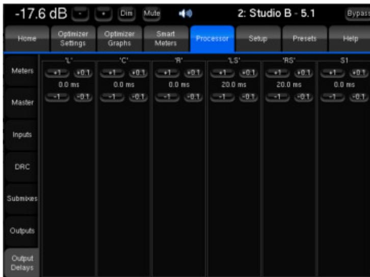
Output delays per channel
